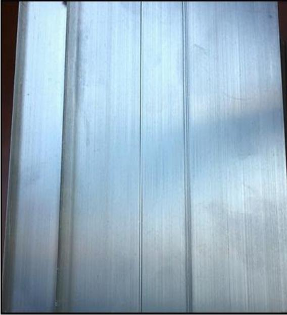
Streaks and tearing(40X). Unacceptable
